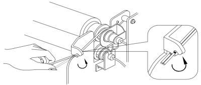
3. Reassemble top cover with retaining screws and do lamination.
